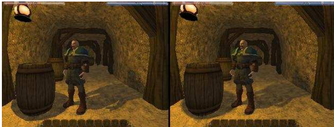
Figure 1.2: Hard vs. soft shadows
